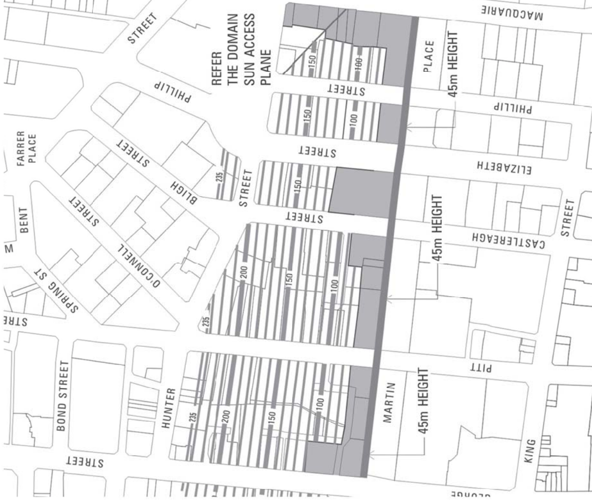
Figure 2. Sun Access Plane Controls (Martin Place) Source: City of Sydney DCP 2012, Section 5, Figure 5.29
